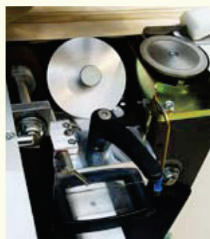
precision glue application, ad- justable to veneer species and throughput speed
