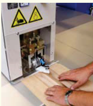
optic-controlled automatic infeed for efficient charging
