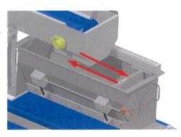
The amount of sprinkle coming out of the hopper is controlled by a knob controlling the gate valve.
