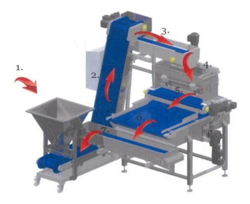
If the sprinkling basket is empty (the state of sprinkle is below the minimum state), then after starting the machine in the refilling basket, the pneumatic actuator will open the gate valve so that the sprinkle goes to the inclined conveyor "Z" (No. 2), which will transport the sprinkle to the top of the sprinkler with the help of a belt with baffles. The gate valve will open and close automatically until the sprinkler basket is filled.
