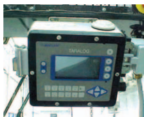
Taralog recording unit located on board of SOILMEC drilling rig recorded diagrams
