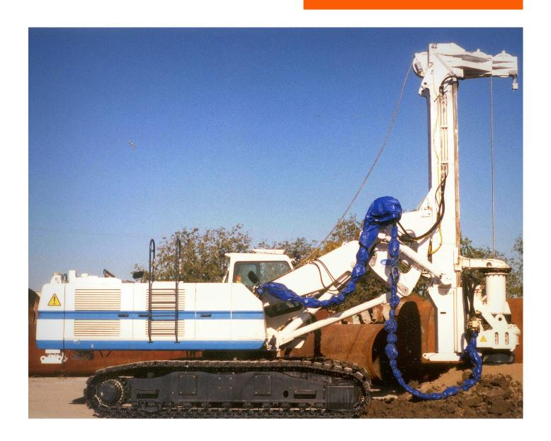
Low Head Room Hydraulic Rotary Rig SR-50
