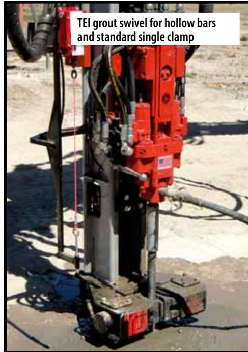
TEJ grout swivel for hollow bars and standard single clamp
