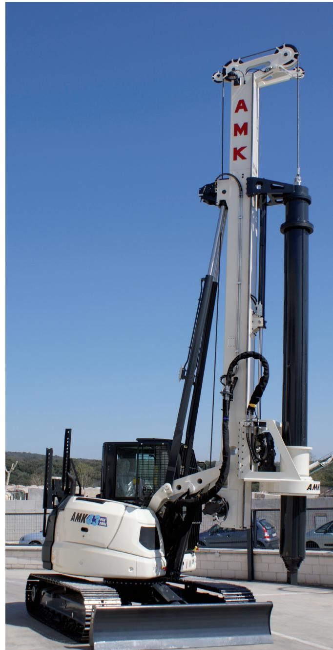
Closed type rotary head, bearings and gears in grease bath with seals and dust protection.
