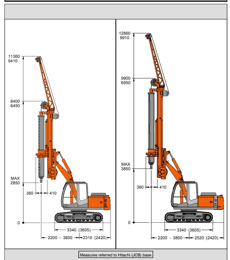
EK60 CFA CFA Piling EK60 LCFA
