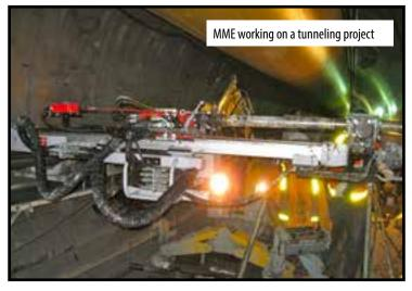
The MME is a lightweight drill for excavators 5-10 tons, incorporating many of the same features as the much larger HEM. The MME uses the same aluminum feed system as the man-portable drills. In this way many contractors consider the MME to be their "outside" drill while the man-portable drill is the "inside" drill. Using TEI's patented drifter technology the MME is an excellent tool for installing micropiles, soil nails, teibacks, rock drilling and the installation of the popular hollow bars.
