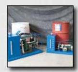
The oil injection system is a self contained, air-actuated positive displacement system. It comes equipped with either a 7 gallon reservoir with sight glass infinitely variable from 0-1 GPH or a 22 gallon reservoir with sight glass infinitely variable from 0-4 GPH.
