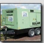
Ideal air match / compressor for LP Drills. 1450 CFM at 200 psi.
