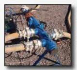
The air manifold connects multiple compressors to a single airline. This manifold is equipped with two 4" and five 3" inlets, two 1" and three 1/4" auxiliary ports, and one 4" outlet.
