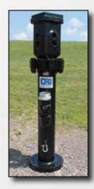
The ratchet attachment is used to supply the LP drill with air when the drill rig is not equipped with air inlet. The ratchet is equipped with the LP's matting bolt flange, shoulder to shoulder lengths of 22" to 60" and can install any Kelly box. To operate, the drill will rotate 360° one direction and 360° the opposite direction.
