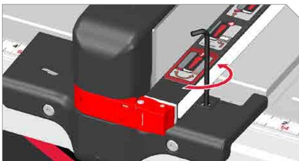
**2** Use a 3 mm hex key wrench to loosen bolt next to indicator lens.
