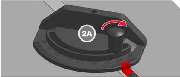
**2** To adjust miter gauge angle, turn lock knob counter-clockwise, and then pivot miter gauge head until red pointer is above desired angle (+/- 60°). Tighten lock knob by turning it clockwise (2A) before making cut.
