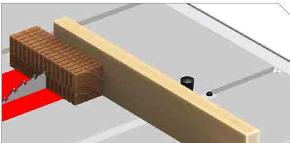
5 As needed, flip workpiece over and make another series of cuts, offset from first set, using same method.
