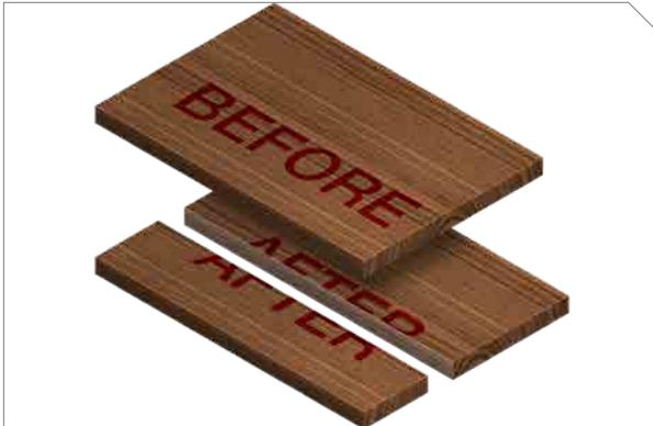
Rip-cutting (cutting with the grain of the workpiece), must be performed with a fence to support and guide the workpiece.
