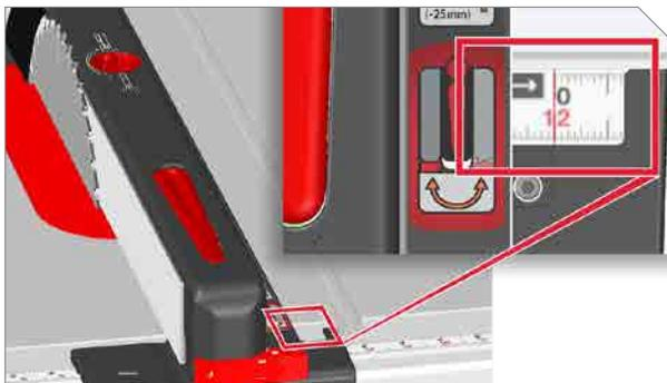
**1** Raise blade fully. Make sure the table is fully retracted. Move fence so its left side rests against right side of blade. If indicator lens reads 0" (0 mm) on ruler, no adjustment is needed. If indicator does not read 0" (0 mm) proceed to next step.
