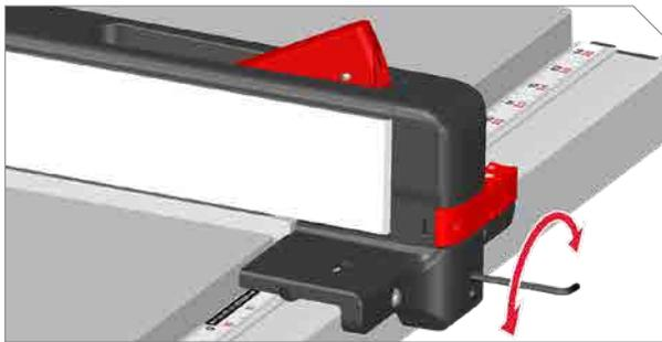
**4** Once fence alignment is done, lock and unlock fence to make sure it is still tightly secured to rail. If fence slides while locked, or feels loose, use a 3 mm hex key wrench to tighten screw on front of fence.
