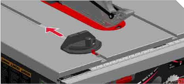
**1** Slide the miter gauge into either miter slot in table top.
