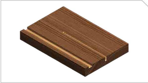
Groove cuts are like Dado cuts and used to create a slot or trench in the surface of the workpiece. However, unlike Dado cuts, a groove is cut parallel to the grain of the workpiece.
