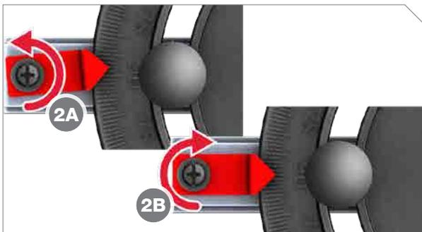
**2** Check that the angle marker is set at 90 degrees. If adjustment is needed, use a Phillips head screwdriver to loosen screw (2A), adjust angle marker to 90 degrees (2B), and re-tighten screw.
