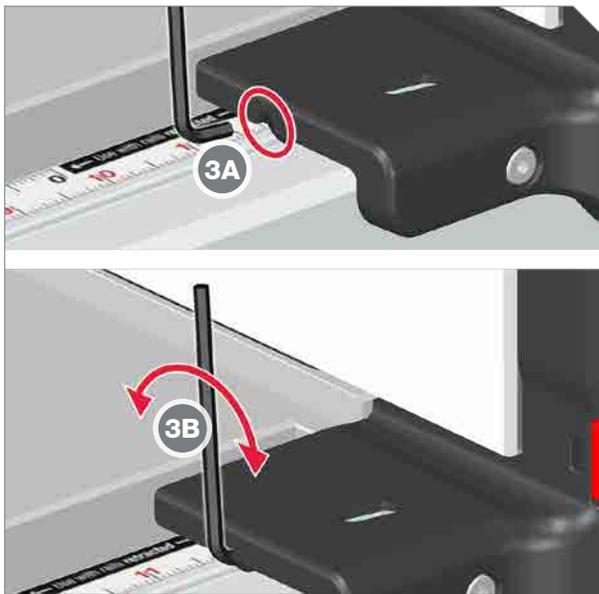
**3** Insert 3 mm hex key wrench (3A) at an angle into hole in left side of fence head. Rotate screw (3B) clockwise to shift fence left, or counter-clockwise to shift fence right. Lock fence and check alignment. Make further adjustments as necessary. When fence is parallel to the miter slot, tighten screw in top left side of fence head. (Reverse Step 2)
