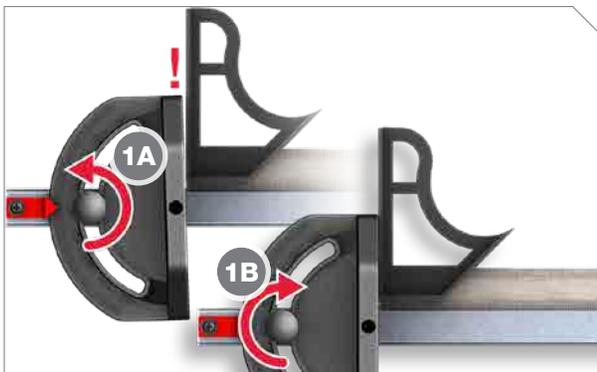
**1** Loosen handle (1A). Use a combination square to ensure that bar and gauge are perpendicular. Tighten handle to lock head (1B). Recheck alignment and make further adjustment as necessary.
