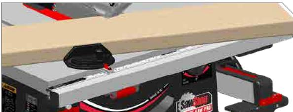
Cross-cutting (cutting perpendicular to the grain of the workpiece) is performed using a miter gauge. The miter angle is indicated by the scale below the pointer.
