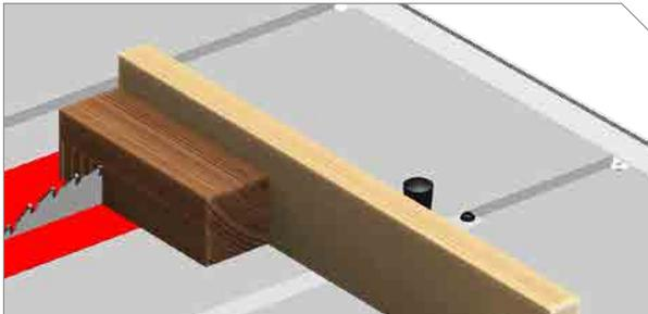
4 Make a series of evenly spaced cuts along workpiece, moving workpiece over slightly between each cut.
