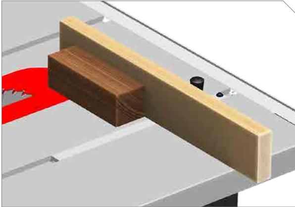
1 Adjust blade elevation to the desired grooving depth.
