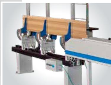
Vertical hopper feeder for moldings 3000 / 4000 / 5000 / 6000 mm.
