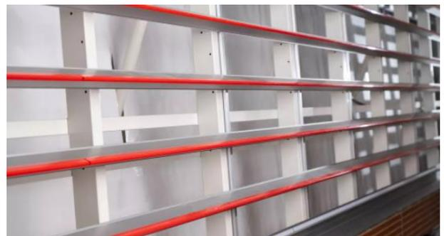
The absolute parallelism between the upper guide rail and the centre and roller support ensures cutting precision for many years.
