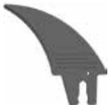
Both the riving knife and the blade guard spreader are designed for 10" blades and have a thickness of 2.3mm. Only use 10" blades with a kerf between 2.35mm and 3.5mm, and with a blade body between 1.8mm and 2.1mm.
