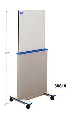
The Adjustable Height Barrier allows the user to position the clear pb at any level between 45.25" and 74". By use of an internal counter balancing mechanism, the clear pb can be moved up or down with minimum effort.
