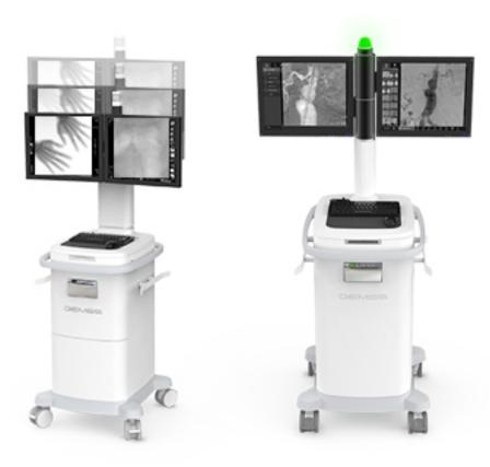
Two LCD monitors can move upward and downward with a driving system, further enhancing users' convenience.
