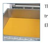
The square press creates uniform, rectangular fat and pastry blocks. The pressing time is adjustable. Available in Electronic version as well. Block size is 43 x 43 cm.
