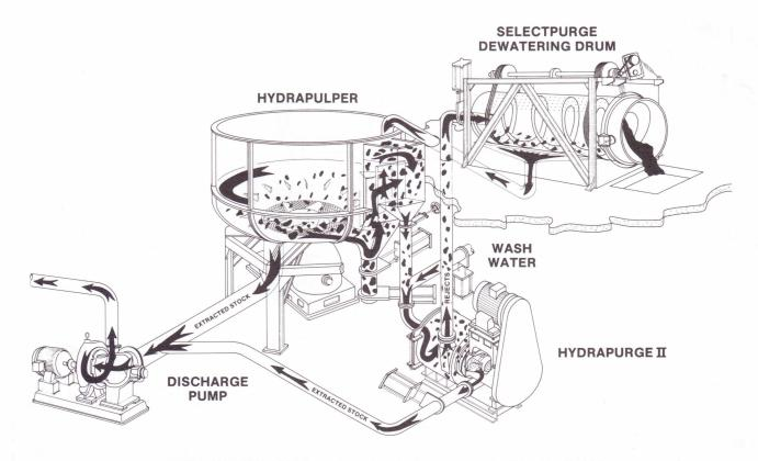
NOTE: This schematic illustrates one method of connecting the Hydrapurge II to the Hydrapulper. The Hydrapurge II can also be connected directly to the Hydrapulper tub, or a trashwell or other junk removal device.
