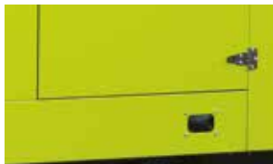
Opening for fuel pipes
