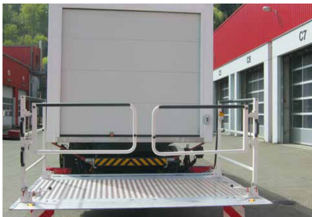
Tail gate with railing and roll stop at the end
