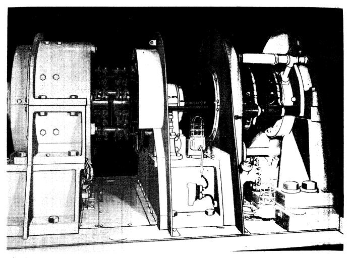
When the exciter housing has been rolled away, all parts that require occasional attention are fully accessible. Ample room is provided around the commutator for changing brushes.
