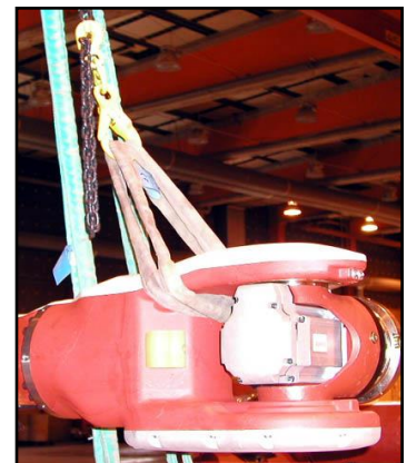
Figure 16. Lifting using a lifting strap.
