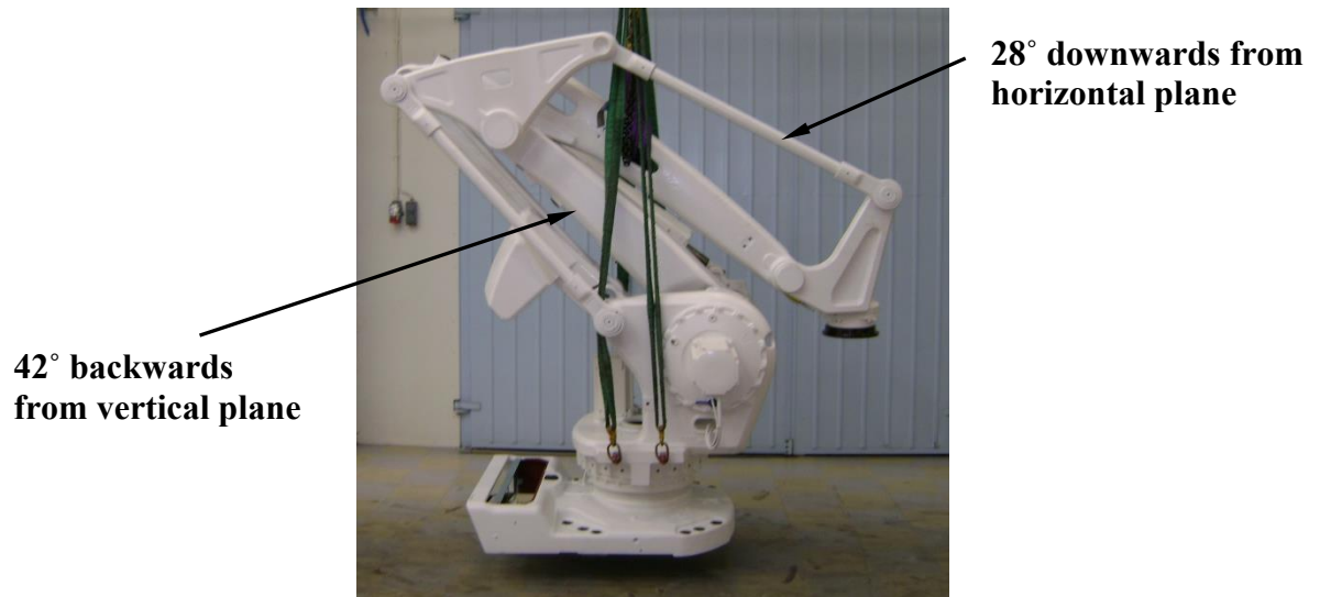
Figure 13. Approved lift position -IRB 760
