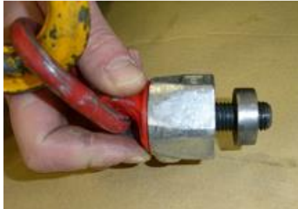
Figure 3. Spacer in WRONG position.
