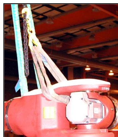
Figure 19. Lifting using a lifting strap.
