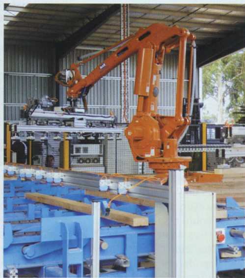
■ Robotic timber sorting system in operation.
