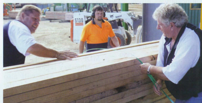
■ Fenning staff strapping timber stacked by the robotic system.
