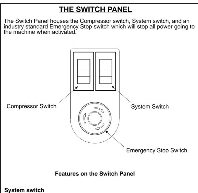
When activated the system switch will operate the motors in order to begin the creasing sequence.
