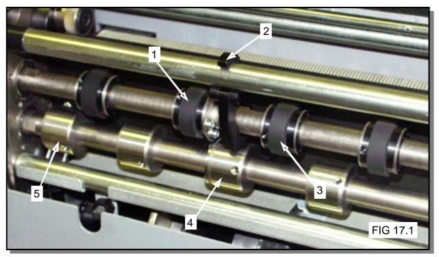
Demonstrates a typical set-up for perforating sheets. Fig 17.1
