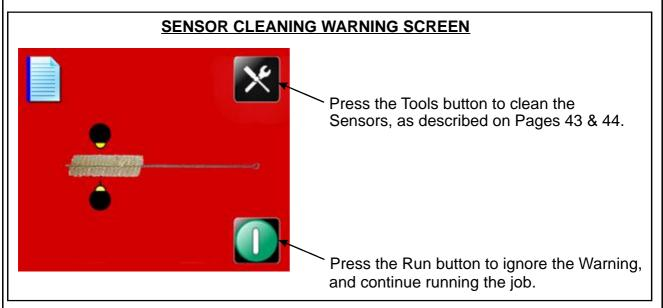
2. The Clean Sensor, Error 65 warning screen, shown below, will appear if the strength of the Lead Edge Sensor Beam is allowed to get down to about 25%. The Lead Edge Sensors should ideally be cleaned before this warning screen appears.
