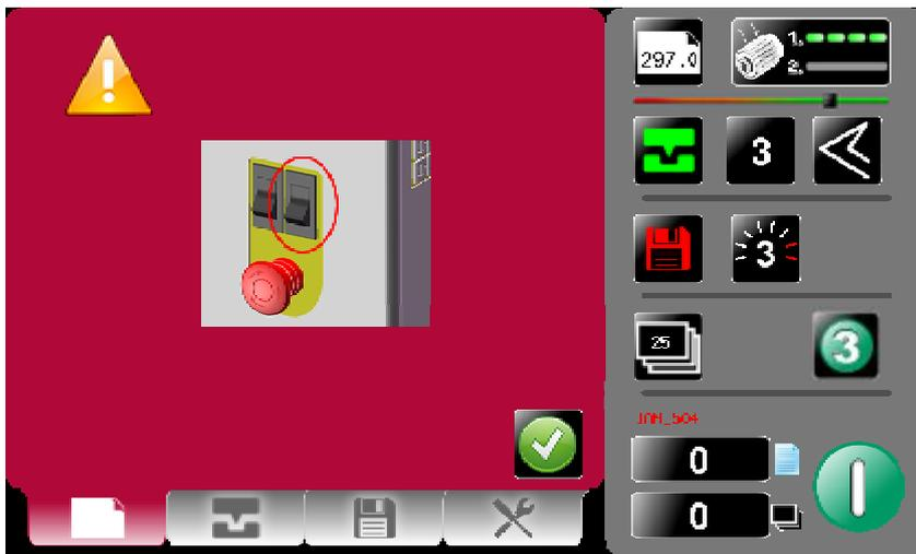
Push System Switch down to start the machine.
