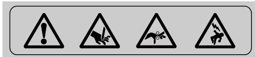
**Do - be aware of any finger traps and rotating parts when operating the machine.**
