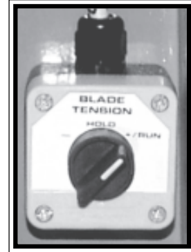
(2) Blade tensioning switch in the tension or run position.
