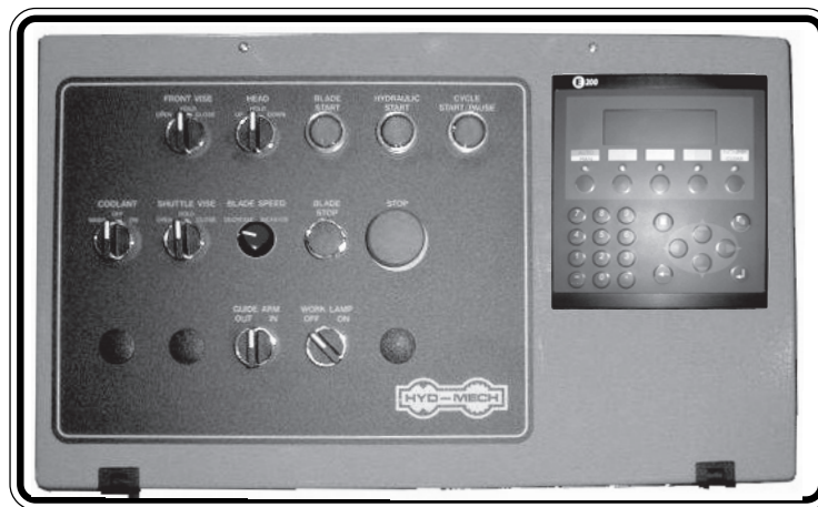
Operator Control Console.
