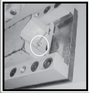
H-18 idler wheel tension slider (one at both ends).
