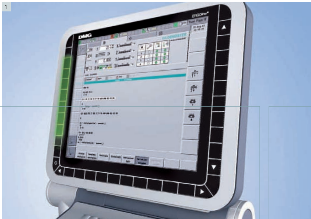
11| 19" screen with DMG SOFTkeys®: Customizable hotkeys for frequently used screen selections or operational sequences
