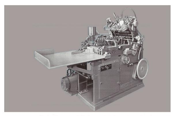
The machines are suitable for manufacturing pockets with side seam gumming, gumming (right-hand side) with outer side flap an centre seam gumming as well as pockets with outer side flaps an powder-proof folding.
