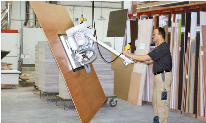
VacuMaster Multi for swiveling wooden boards by 90°
