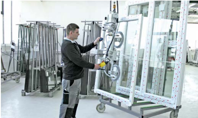
VacuMaster Window for rotating and palletizing windows
