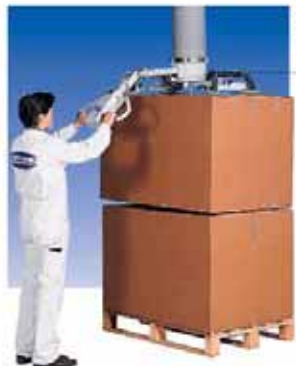
JUMBOERGO with swivelling controls for high stacking.
