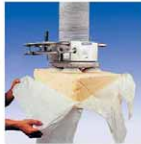
JUMBO SPRINT , made of stainless-steel, fitted with vacuum head for butter/cheese.
