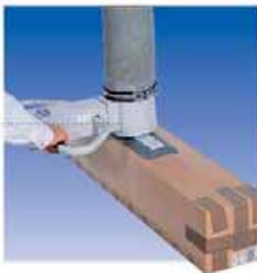
JUMBOERGO with long rectangular vacuum head for narrow loads and parcels.
