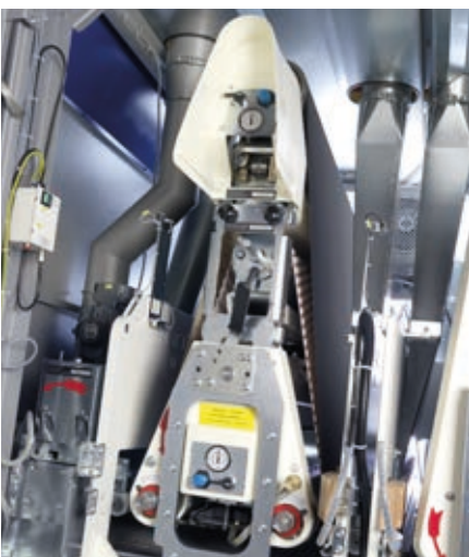
Longitudinal sanding unit (with pressure segment belt)
