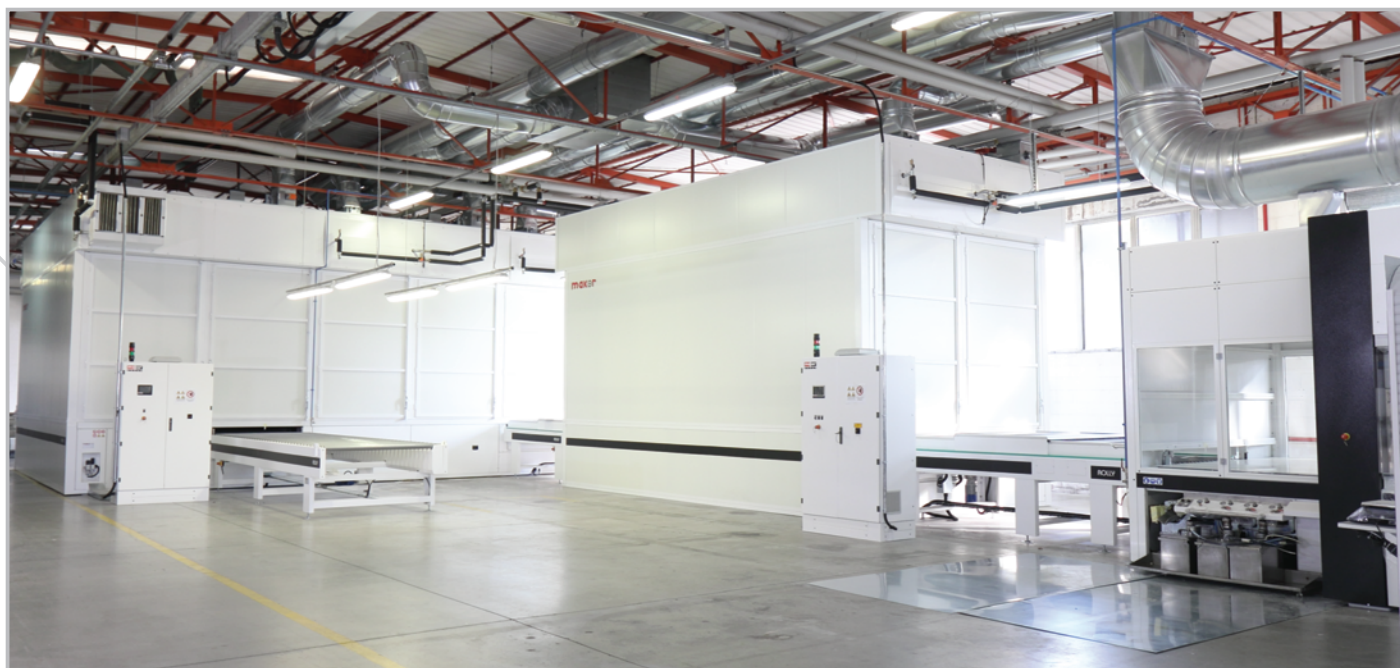
Plant for glossy lacquered doors - 2 stages flash-off oven - 6 stages drying oven
