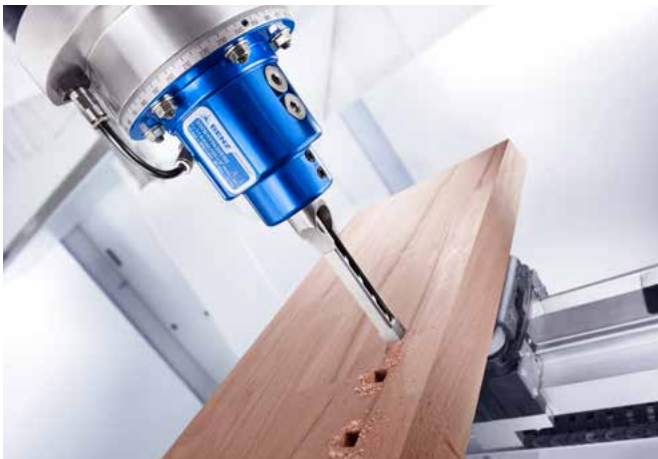
Stake holes for steps
