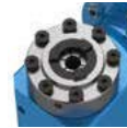
Centring Ø40 (TK Ø52 - 8x M5)/ collet chuck holder ER25A per DIN6499 with internally located clamping nut
