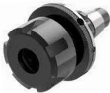
Collet chuck holder with externally located clam- ping nut per DIN6499 Clamping range ER 25 \varnothing 2– \varnothing 16 ER 32 \varnothing 2– \varnothing 20
