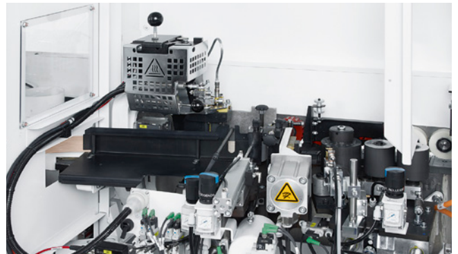
Gluing units for safe hot-melt glue application
