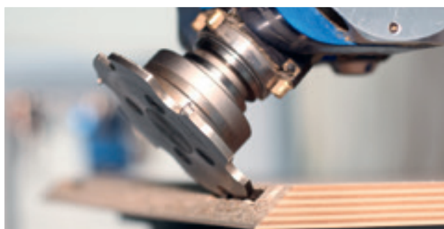
Cutting recesses for connecting fittings
