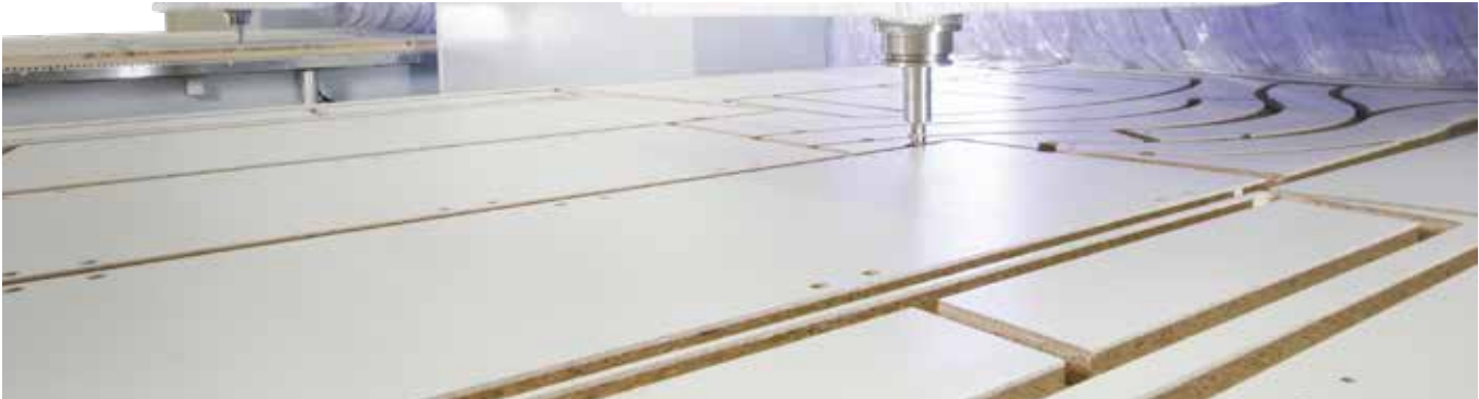
Nesting processing of panel materials: waste-optimized cutting to size and processing in the surface
