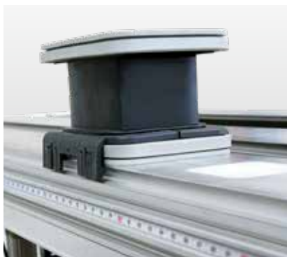
Measuring tape for positioning the suction units.
