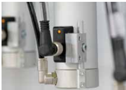
Electronic cylinder surveillance Improved safety by electronic surveillance of all stop cylinders.
