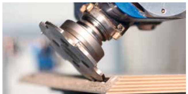
Cutting recesses for connecting fittings
