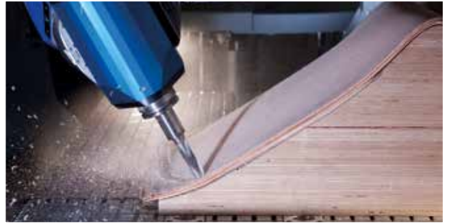
Routing of shaped wood
