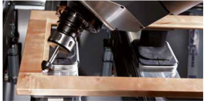
Square corner cutting for a glass rebate
