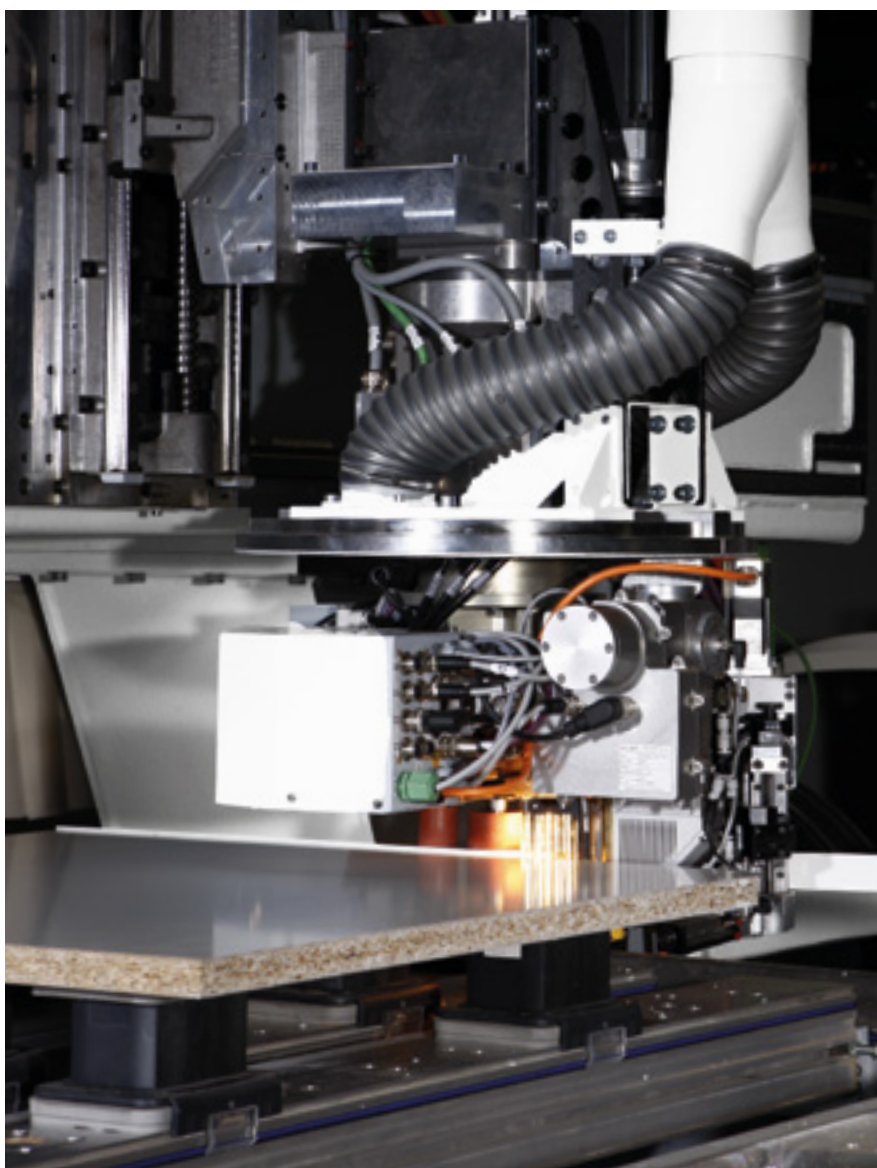
laserTec shaped component edging with zero joint
