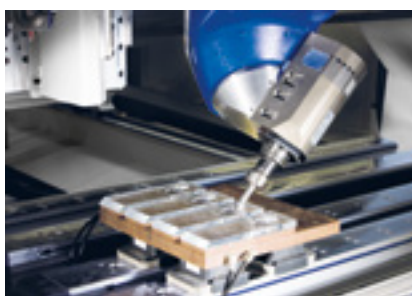
High-gloss trimming of acrylic parts
