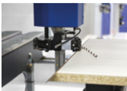
Scraping of mitered edges
