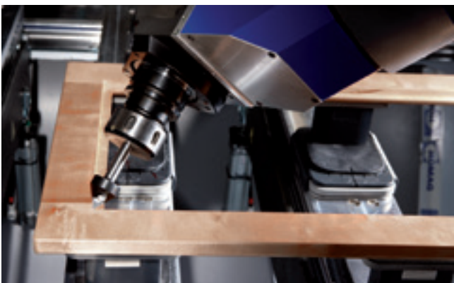
Angular cutting of a glass rabbet corner
