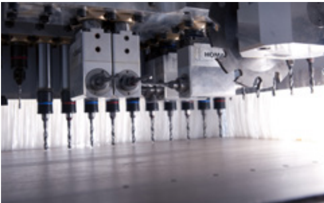
High-speed drilling technology with groove saw
