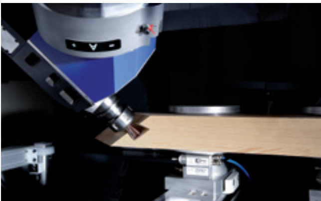
Routing a burr connection for jamb/rail designs
