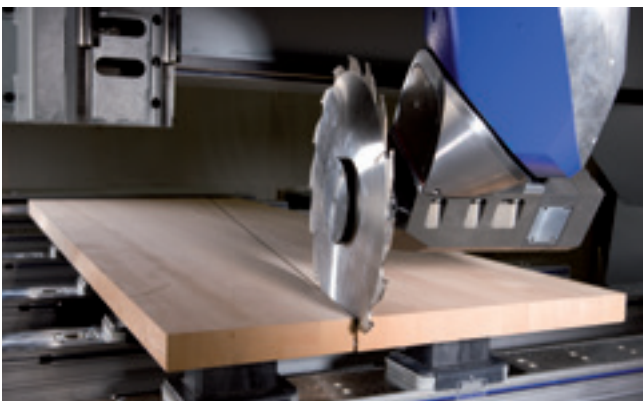
Separating cuts up to 110 mm in height
