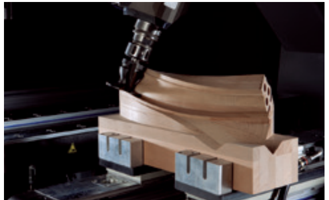
Routing a staircase handrail
