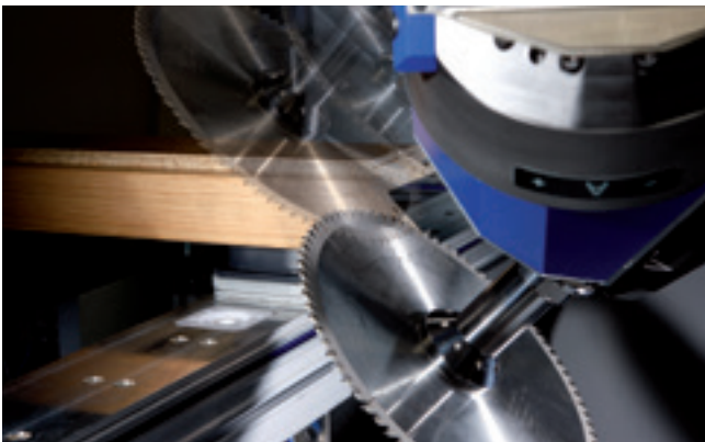
Precise and tear-free miter cuts
