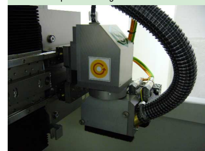
Disc depanelling module with vision system
