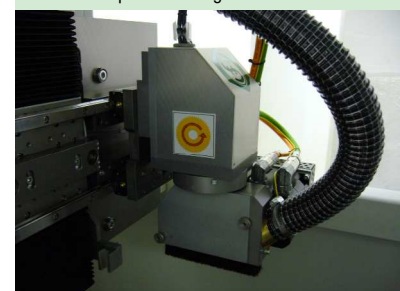
Disc depanelling module with vision system
