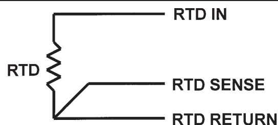
FIGURE 10-2. Three-Wire RTD Configuration.
