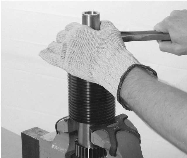
Figure 51 — Using spindle wrench to remove the spindle nut.
