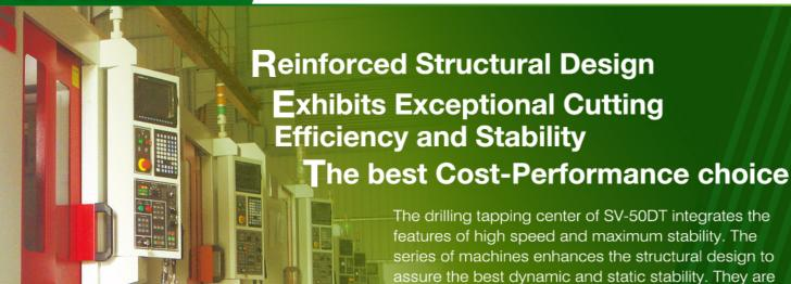
equipped with a 12,000rpm high speed spindle, combined with 48 m/min. rapid traverse rate on three axes making an optimistic integration for high speed,
