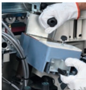
Quick locking system for glue pot change
