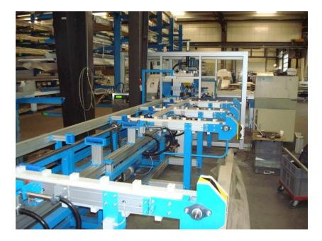
This makes it possible to insert profiles in about 10 warehouse positions against 6 pieces in an existing set-up. 4 new tires with partly new cams. The 4 minitek 90x90 support profiles must be extended approximately 10 to 20 cm.
