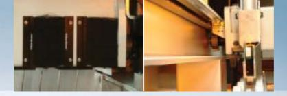
Residue cutting device for cutting residues. The clamps travel into the recessed pressure beam.
