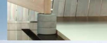
The pneumatically controlled angle pressure device holds workpieces securely in position and thereby ensures a precise cut, even in the case of long workpieces.
