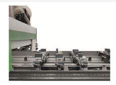
The system, depending on the programming of the worktops on the software interface, indicates to the user the direction of movement of each worktop and carriage, and signals via green and audible LED the position reached with an error of  $\pm$  /  $\pm$  1.5 mm.
