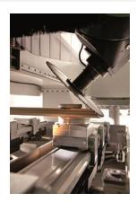
For optimum dissipation of the heat produced by the electrospindle during machining, a coolant cooling unit is used.
