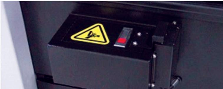
» **Parts Catcher:** Air operated swing plate type parts catcher. Parts are transferred to an enclosed bin mounted outside the sliding access door. The kit includes an air pressure regulator, dryer, and lubricator.
