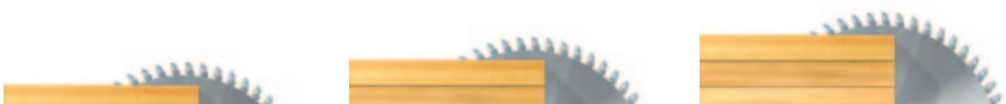
The main saw blade projection is automatically adjusted by the numerical control in relation to the thickness of the stack to be cut, thus obtaining the best cutting quality under any working condition. On the Sektor 450 K1 model the saw blade projection is automatically adjusted in two steps.
