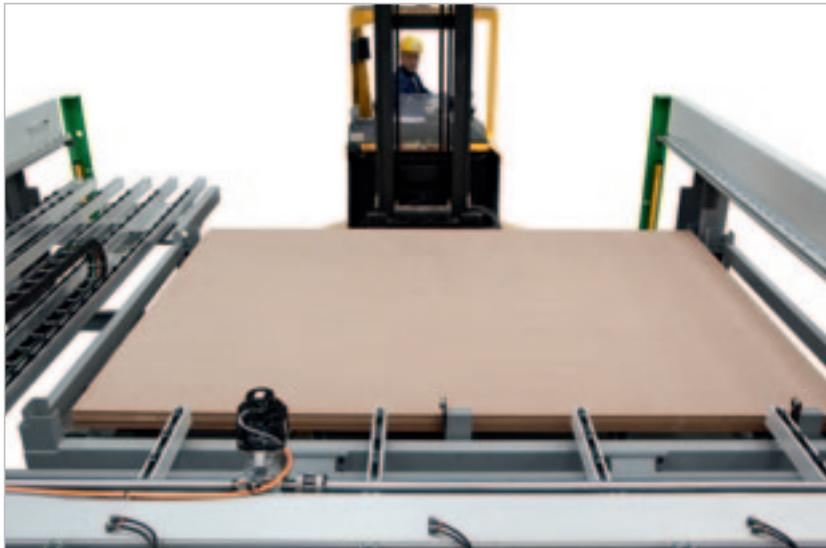
Lift table compact and integrated for automatic loading of panels, allows the loading of stacks of panels up to 500 mm directly on steel profiles. Possibility to install the lift table as retrofit.
