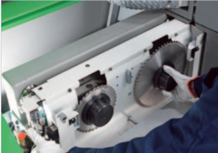
“Quick change” system for fast saw blade change (patented).
