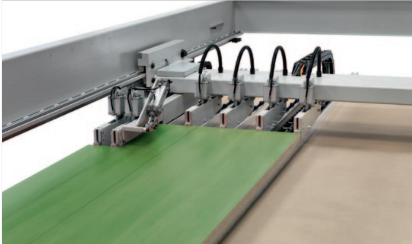
With optional device Twin Pusher it works like having two cutting lines on the same machine. It allows simultaneous cutting phases thus dramatically reduces working cycle time.
