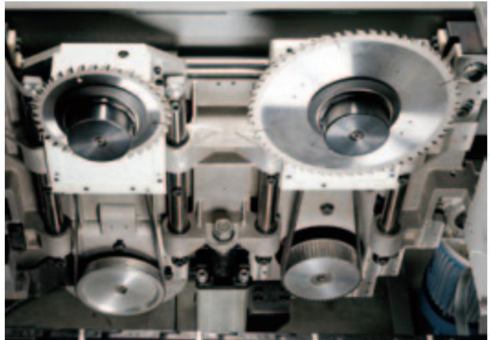
Independent raising and lowering of main saw blade and scoring saw blade is due to system that guarantees precision and rigidity to obtain a high cutting quality.
