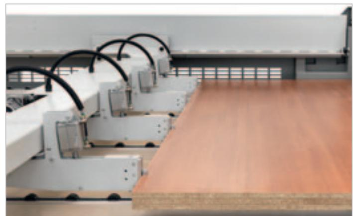
The pusher carriage for precise and fast panel positioning is driven by a brushless servomotor.
