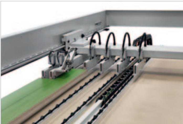
**Staggered cross cutting of narrow strips.**
