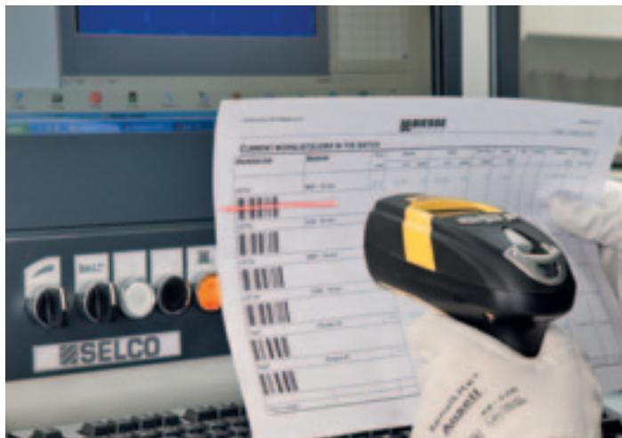
**Barcode scanner:** to automatically recall the cutting patterns and automate the management of reusable cutting pieces.\*
