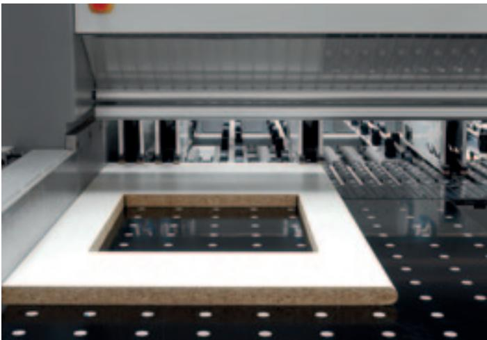
Software to execute window openings on panels. The various patterns can be stored on the numeric control (option).
