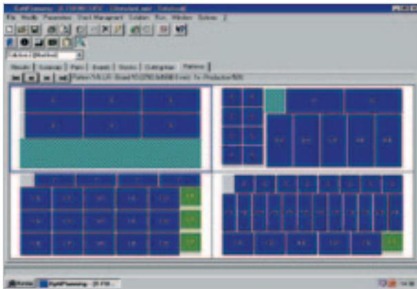
**OptiPlanning:** cutting patterns optimisation software to minimise total machining costs in terms of both effective material cost and sizing times.\*
