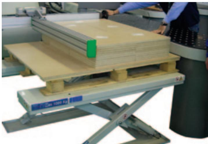
**Hydraulic table to unload on pallet cut panels.** The table has a manually adjustable stop fence, which can be turned over to make the removal of the pallet easier.
