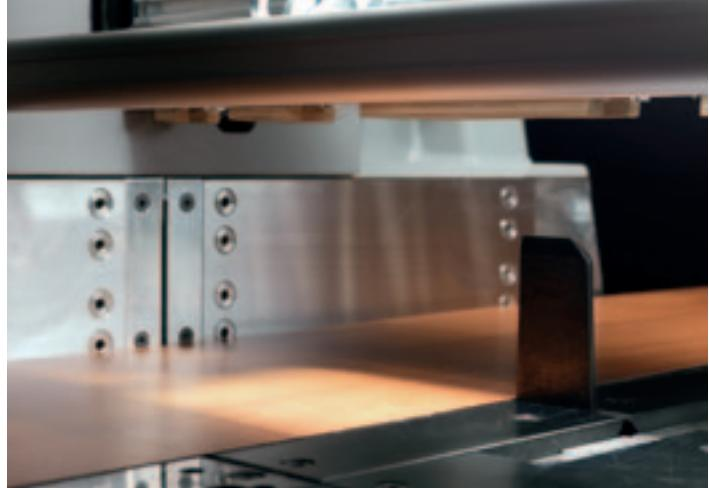
The side aligner is integrated with the saw carriage. It can perfectly align even thin or flexible panels, reducing cycle cutting time.
