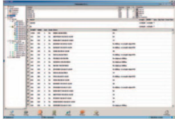
**Quick Opti:** simple and intuitive “On board” optimizing software to elaborate cut list directly on the personal computer on the machine.\*
