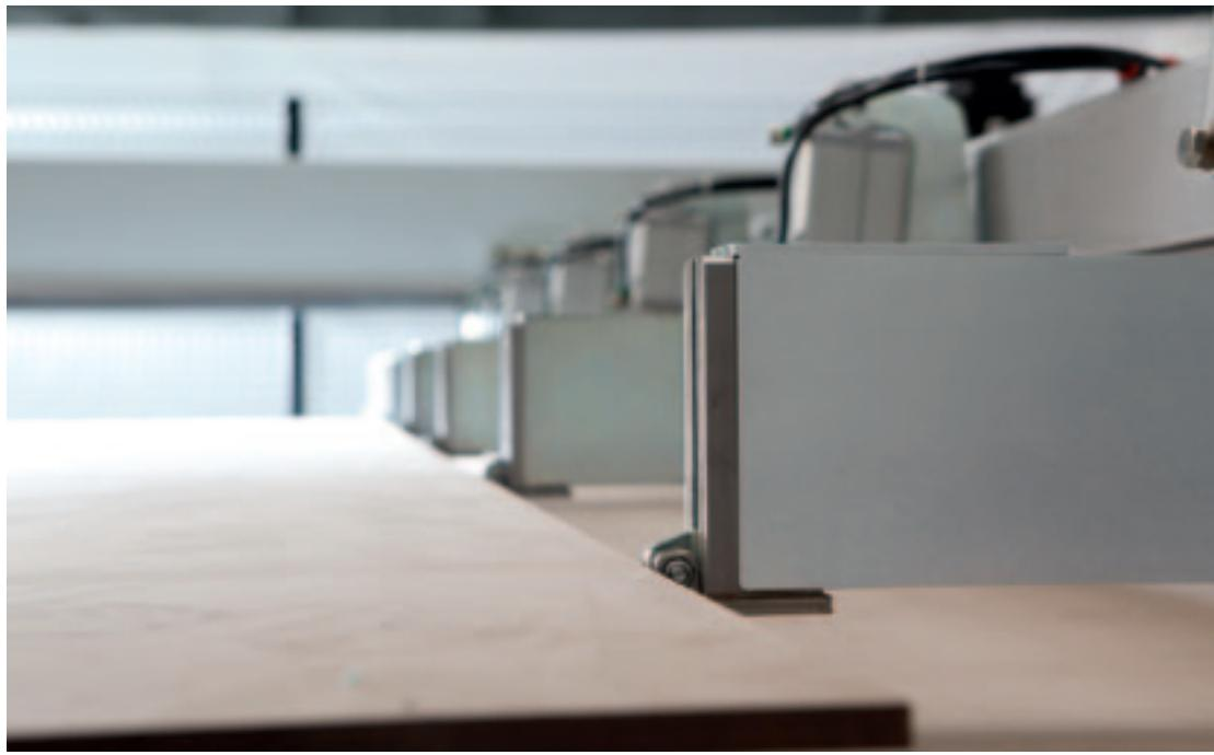
The automatic picking of the panels is executed by the grippers according to the cutting pattern requirement.
