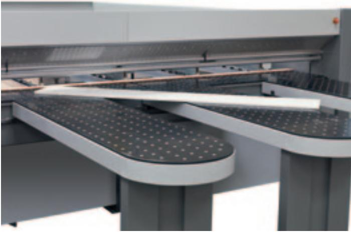
Grippers with special fitting system for cutting stack of panels with overhanging edges (option).
