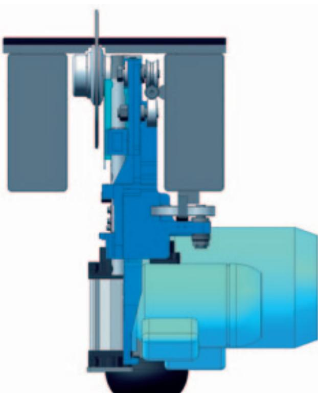
The top guide, positioned right beside the saw blade hub, guarantees the total absence of saw blade vibrations.
