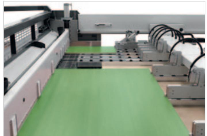
**Cross cutting and rip cutting on the same cycle.** An additional side support permits to cross cut independently strip up to 650 mm wide.
