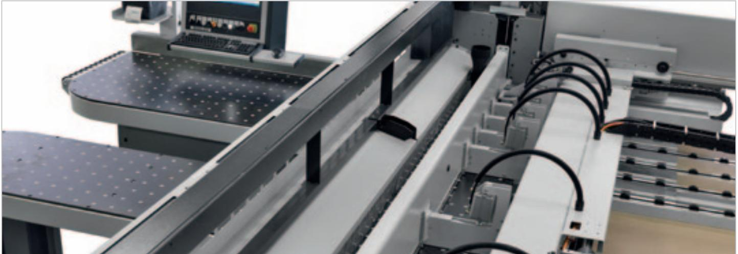
The pressure beam has a single structure for an even pressure on the stack of panels to be cut. The opening is automatically adjusted by the numerical control in relation to the thickness of the stack to be cut, thus obtaining the best cutting quality under any working condition. (Not available on Sektor 450 K1.)
