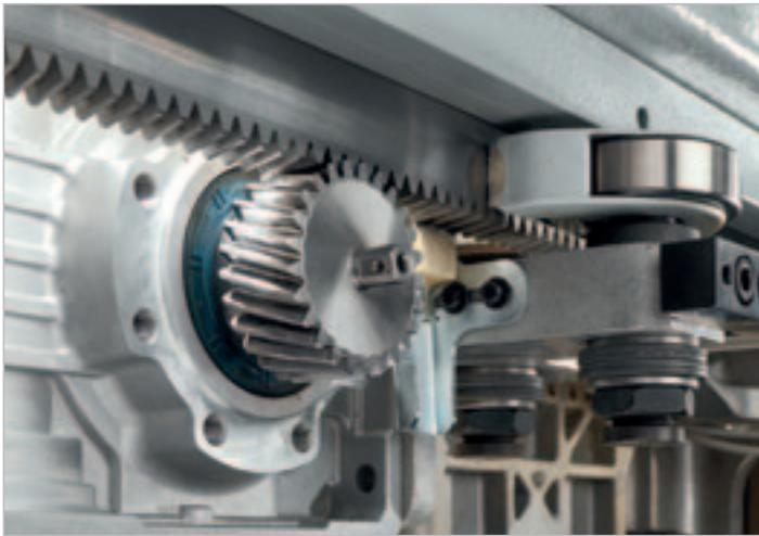
The extremely linear movement of the saw carriage is obtained by an helical rack and pinion system and by a brushless motor.
