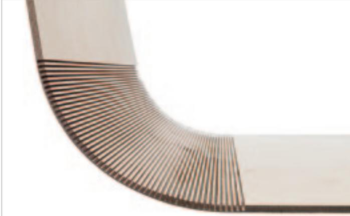
Device for the automatic execution of grooves whose width may be programmed by the numeric control. The groove depth may be manually adjusted. (Electronic adjustment available by request).
