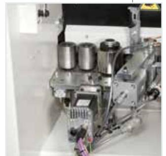
**Pressure roller conveyor with electronic positioning and timed intervention.**
