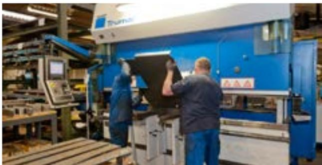
Computer assisted steel plate bending
